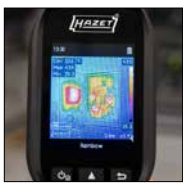
Photo + thermal object image = Fusion Mode
