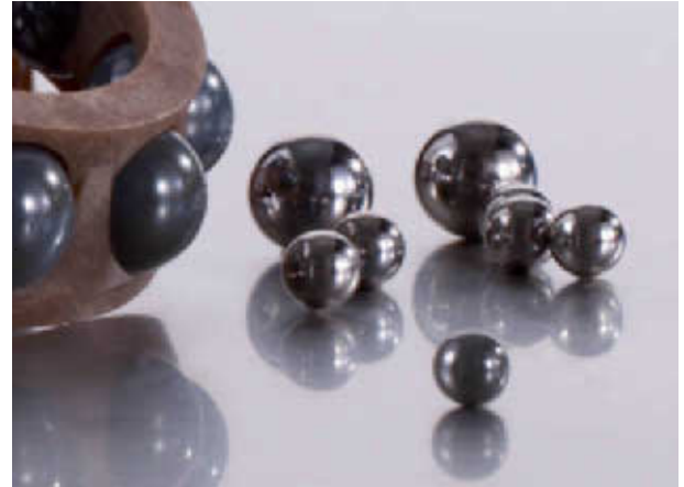
Fig. 6.1: Rolling elements made of Si 3 N 4 and 100Cr6
